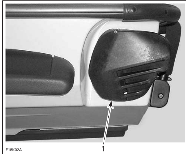
1. Side vane in upper position
