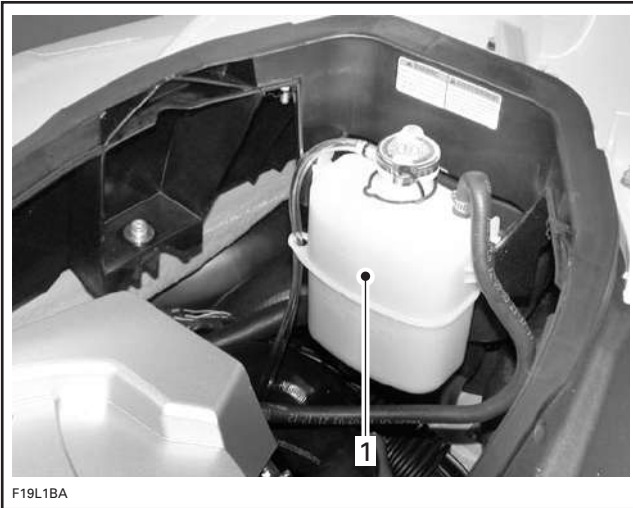
1. Coolant expansion tank
