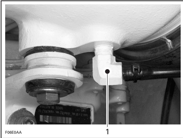
1. Water injection hose
