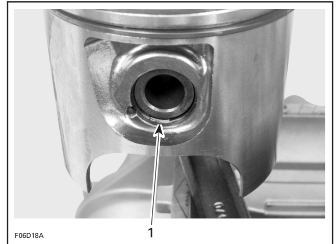
1. Circlip opening at 6 o'clock (at bottom)
